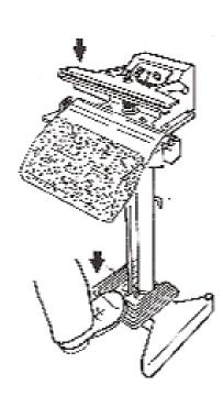
4 THE SEALING TIME IS INDICATED. BY THE SIGNAL LIGHT ON THE TIME PANEL AND THIS AUTOMA-TICALLY CONTROLS THE HEA-TING PERIOD WHEN PRESSING THE FOOT PEDAL.
